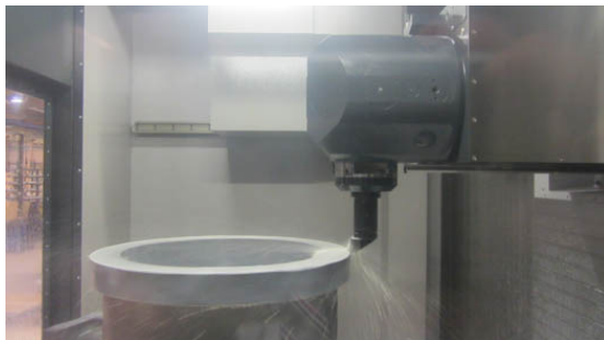
Bild Nr. 01-03 SH_OG-Fraesen.jpg With the SHW machine, the main machining times have been reduced by over 30 percent.
