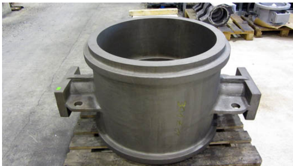
Bild Nr. 01-01 SH_OG-Rohling.jpg Around 650 kg is what the grey cast iron casting of the butterfly valve weighs on the work table of the machining centre.
