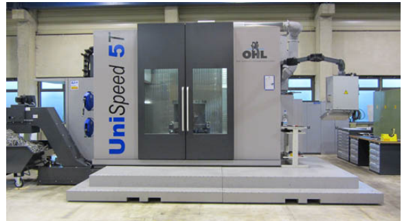
Bild Nr. 01-02 SH_OG-UniSpeed5T.jpg Mill-turning centre UniSpeed 5T from SHW Werkzeugmaschinen with axial lengths of X = 2000 mm, Y = 1300 mm and Z = 1300 mm for machining workpieces weighing up to 6t.
