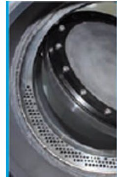
Bild Nr. 01-12 SH_OG-Klappensitz.jpg For reliable pressure tightness of metallic sealing KX Butterfly valves, precise machining of the three times eccentric valve seats is vital.
