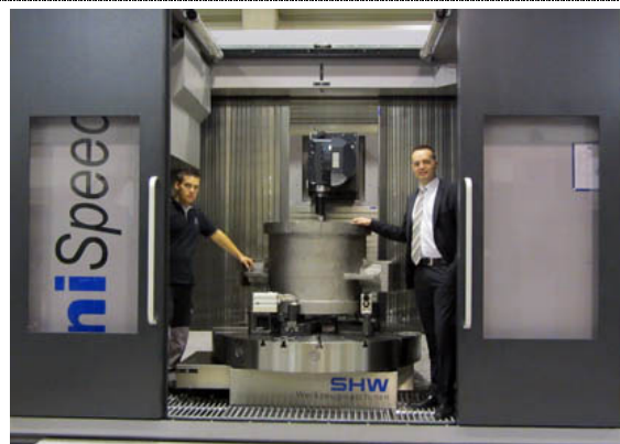
Bild Nr. 01-10 SH_OG-RauSchultheis.jpg A specially developed programming routine machines the different angles in the valve seat from 2 degrees to 22 degrees with the desired result -thanks to close cooperation! (Christian Schultheis, left, Project leader Sören Rau, right, both from OHL Gutermuth).
