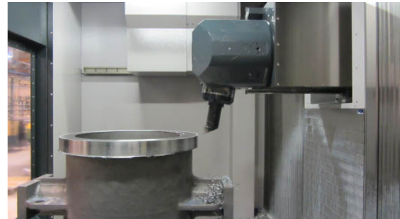
Bild Nr. 01-04 SH_OG-Position.jpg The compact and powerful orthogonal head can reach 64,800 individual positions.
